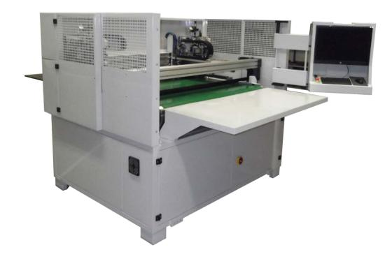
We prepared a new digital version to enrich the **Saturno** range (Saturno 2 and saturno 2.2). This new digital version has a powerful architecture for the management of the user interface and for the external management of CAD / CAM system. The use of a latest generation processor allows now the real-time control of the machines
